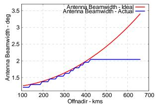
Fig.-2: In order to keep illumination swath constant across range swath, RISAT-1 Antenna beamwidth is being programically controlled w.r.t pointing by controlling antenna illumination along cross track. Figure shows variable beamwidth tracking required ideal beamwidth of antenna upto 420km swath, beyond that swath is controlled by return echo time.
