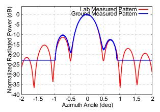
Fig.-7: Comparison of measured Azimuth Antenna Pattern during testing in Lab and after launch ground measurement with a customized measurement setup. Results show a reasonable match upto first sidelobe.
