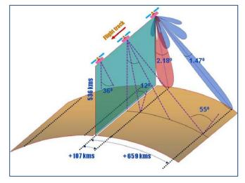
Fig.-1: RISAT-1 Antenna Beam Pointing showing Near and Far beams with variable beamwidth of 2.18 to 1.47 Range swath coverage from 107km to 659km is covered in 61 antenna beams with 10km step at spacecraft roll angle of  $36^{0}$  and nominal flight altitude of 536km.
