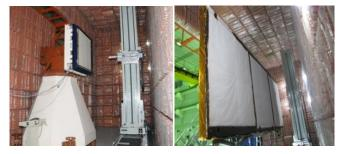
Fig.-3: RISAT-1 antenna test facility (Pulsed PNF) equipped with 3D scanning system. Left side image shows single antenna tile (24 TR elements) under test, whereas, right side image shows full antenna (288 TR elements) being scanned in Pulsed PNF
